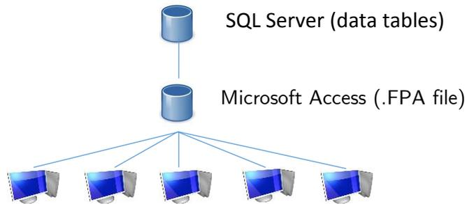
*Figure 9 - SCOPE 5. SCOPE 5 desktop users connect to an FPA file stored on a file server. The FPA file does not contain the data tables, which are stored in the Microsoft SQL Server database. Microsoft Access transparently requests data from Microsoft SQL Server as needed.*
